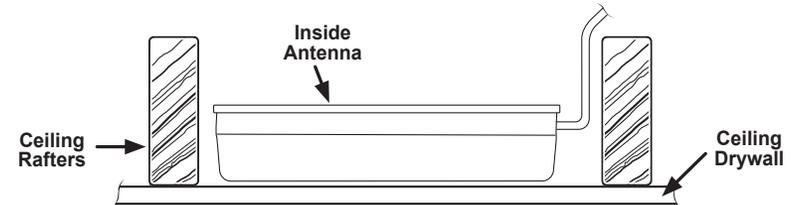
In some cases, multiple Inside Antennas may be required, for instance if you have multiple rooms with poor signal. A signal may be split by using a splitter (sold separately). If using more than one Inside Antenna, a separation up to 75 **horizontal** feet may be necessary between Inside Antennas. See configuration on pages 3 & 4.
