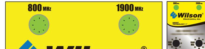
**Note:** If after the initial 15 minutes you are not done with the installation, the Signal Booster can be reset and enter installation mode again by disconnecting and reconnecting the power supply from the Signal Booster.
