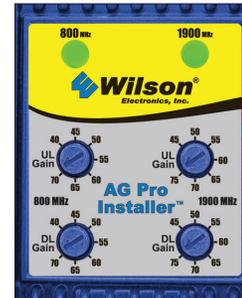
This Signal Booster is supplied with separate uplink and downlink gain controls. **Note:** All gain controls should be set to maximum. If you have green lights, the installation is complete.
