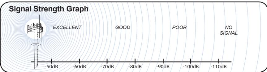
Signal readings usually appear as a negative number (for example, -86). The closer you get to zero the stronger the signal (see graph above).
